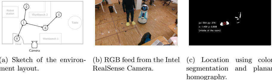
Fig. 1: Environment for ER scenario, including the environment layout, a frame where both robot and human are in position 3 (next to Workbench 1), and the segmentation and homography, used to locate the human in the environment.
